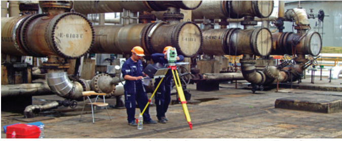
Laser surveying in action at the Sisak refinery using a Leica Total Station.
