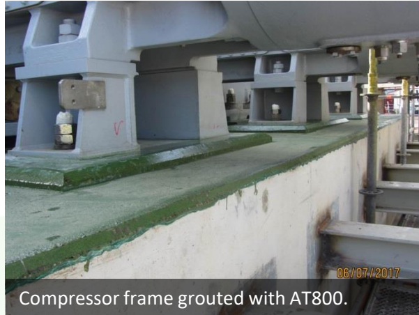
Cylinders supports with Alphatec® Epoxy Grout (in green).
